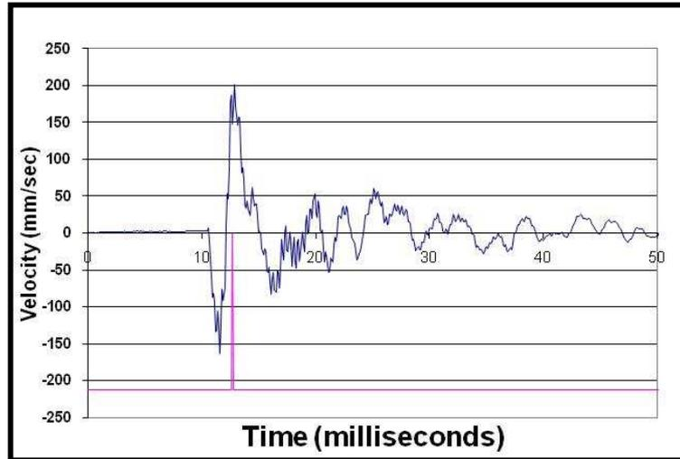
The result for this particular cable bolt calibration test showed that good mechanical admittance and structural stiffness has been achieved throughout the 4m cable bolt length for a full column grouted bolt (see Figure 6) during testing.
