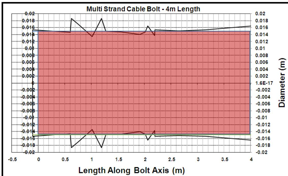
The above results were compared to the results for the semi controlled partially grouted twin strand cable bolts (see Figure 7 – 6m long twin strand cable bolt proposed grouting between 5 and 6m). This showed a significant reflection and lower structural stiffness.
