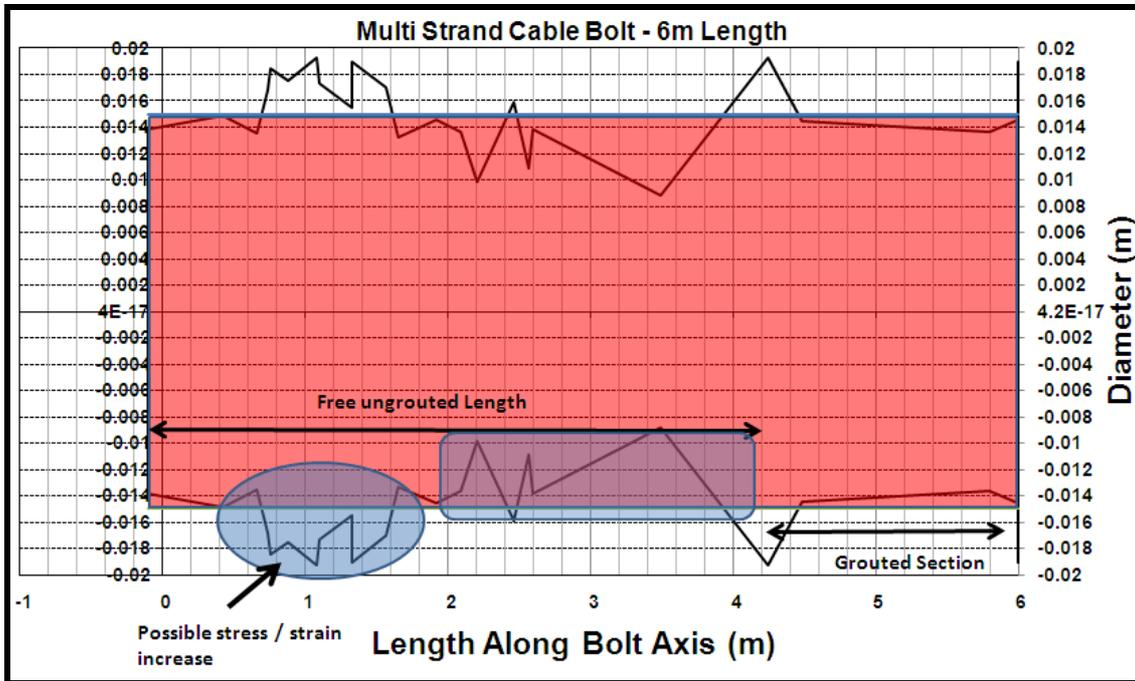
47 Bolts were tested (15 Posimix Bolts and 32 Cable bolts). Of the 15 Posimix bolts tested four showed signs of overstressing (i.e. bolts subject to ground deformation – see Figure 8) and of the 32 Cable Bolts tested three showed signs of overstressing.
