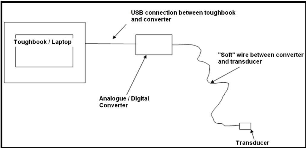
Figure 2 – Transducer and tapping device used to excite (generation of seismic signal) the element.
