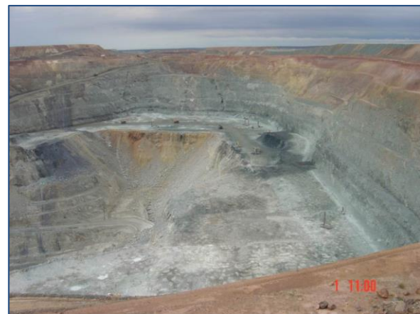
Open cut final bench blast preparation.
