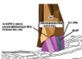
Figure 2 Cross section looking West – South west, showing fill height to be maintained during 6z1 A-Pillars extraction
