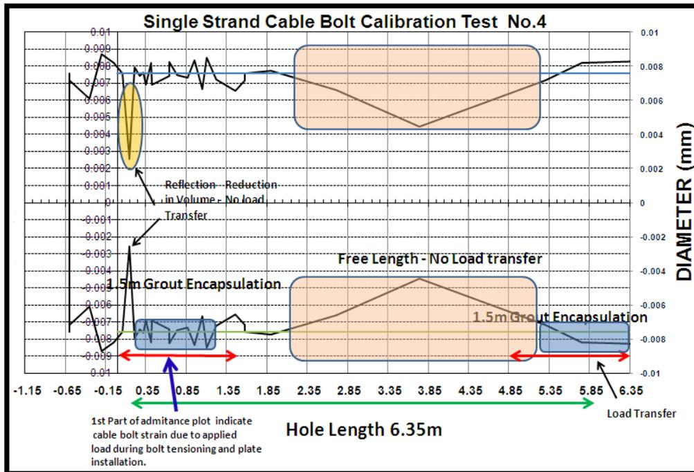
**Figure 6 - Two dimensional graph showing structural stiffness of rock reinforcement element with diameter used as a guide**
