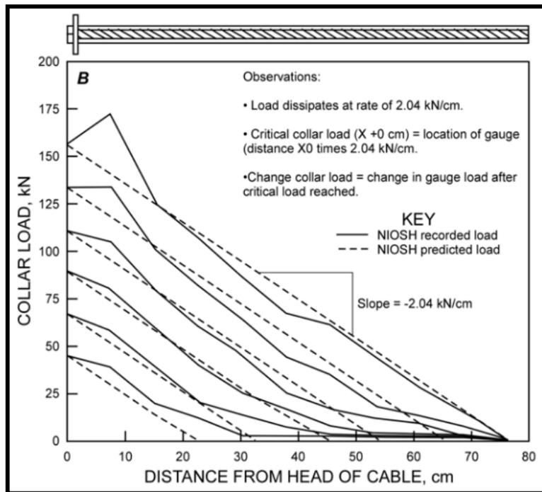
**Figure 10 - Collar load plotted against A, microstrain (load profile curve) and B, distance from head of cable (load correlation curve, Martin et al.(2004))**
