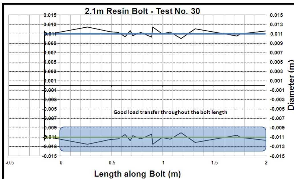
**Figure 8 - Two dimensional graph showing good embedment achieved along the length of the 2.1m resin anchor installation**
