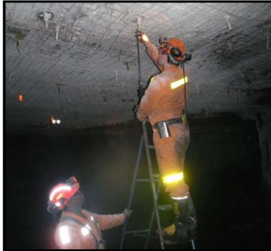
**Figure 3 - Photo showing transducer (vertical) held at the end of bolt (i.e. collar of hole) at Mandalong Coal Mine**
