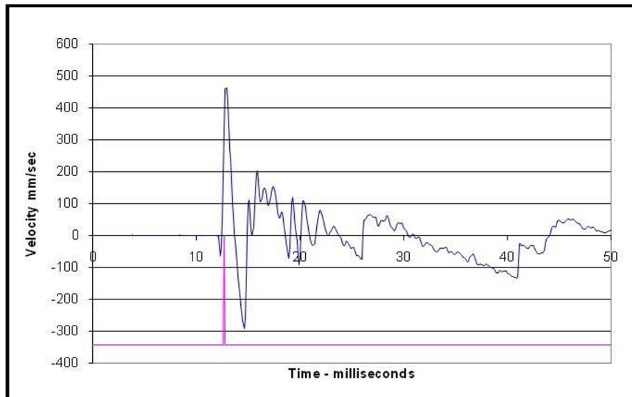
**Figure 5 - Diagram showing valid seismic signal obtained by transducer (geophone)**
