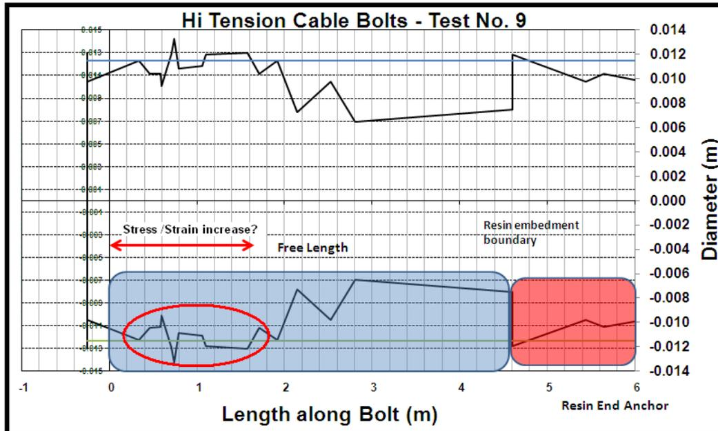
**Figure 9 - Two dimensional graph showing confirmation of end anchor resin embedment and possible stress / strain increase in close proximity of hole collar**
