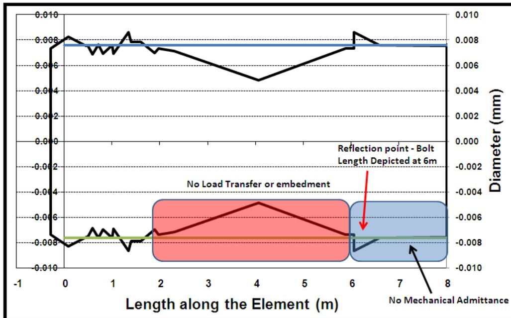
**Figure 7 - Two dimensional graph showing confirmation of twin stand cable bolt 6m length following initial 8m input parameter**
