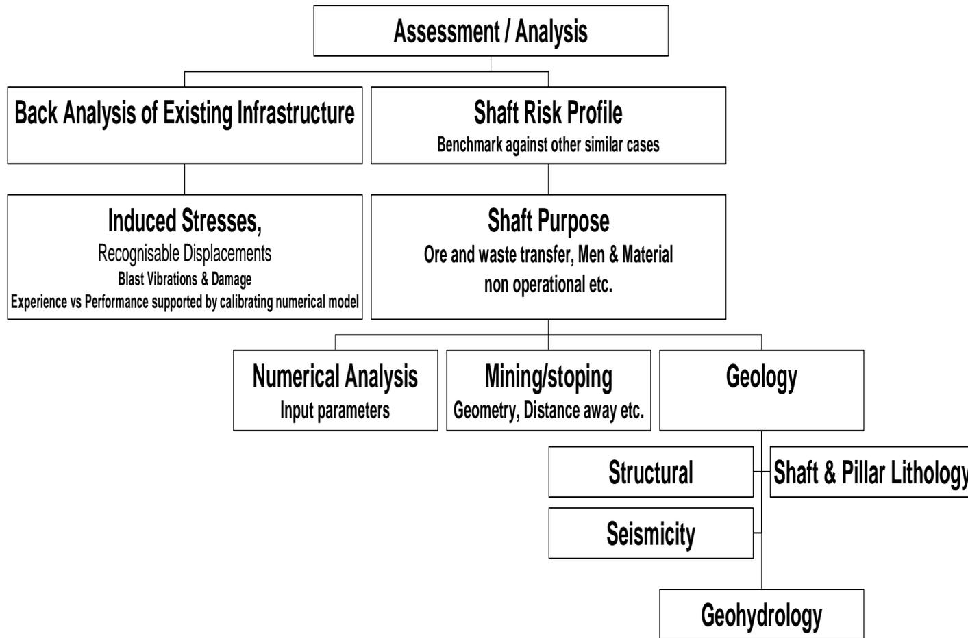
**FIG 3: Example geotechnical process map of shaft pillar design.**
